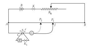
A battery B, a rheostat ( $R_h$ ) and a key K is connected across the ends A and B of the potentiometer wire such that positive terminal of battery is connected to point A. This completes the primary circuit.
